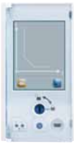
Earth fault tripping curve preview
